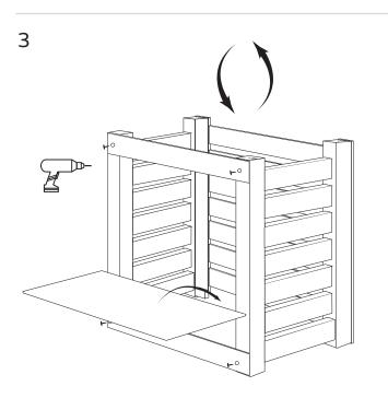
Flip the cover back to the correct position and screw the top and bottom wood for support. Add the bottom support where chiller will be placed.
