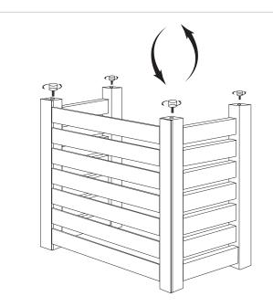
Flip the cover upside down and install provided rubber feet by screwing it into the base.
